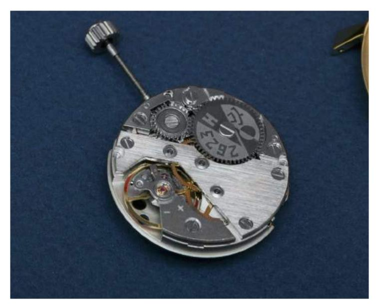
The Calibre 2623 is extremely close to what was found in the original 1970 watch. This hand-wound movement, with 24-hour display, is by no mean a high-end, Haute Horlogerie piece. It was created to be robust, functional, easy to service and durable. This calibre runs at a slow frequency of 2.5Hz and boasts a 42-hour power reserve. It adjusted in 4 positions and should run at ±10 seconds/day.
