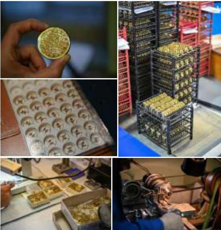
Almost the entire movement is produced in-house, from the wheels to the bridges, the main plates, the pinions and even the hairspring – it is extremely rare to see this in a manufacture, even in Switzerland. The movements are then assembled and tested, before being cased.
