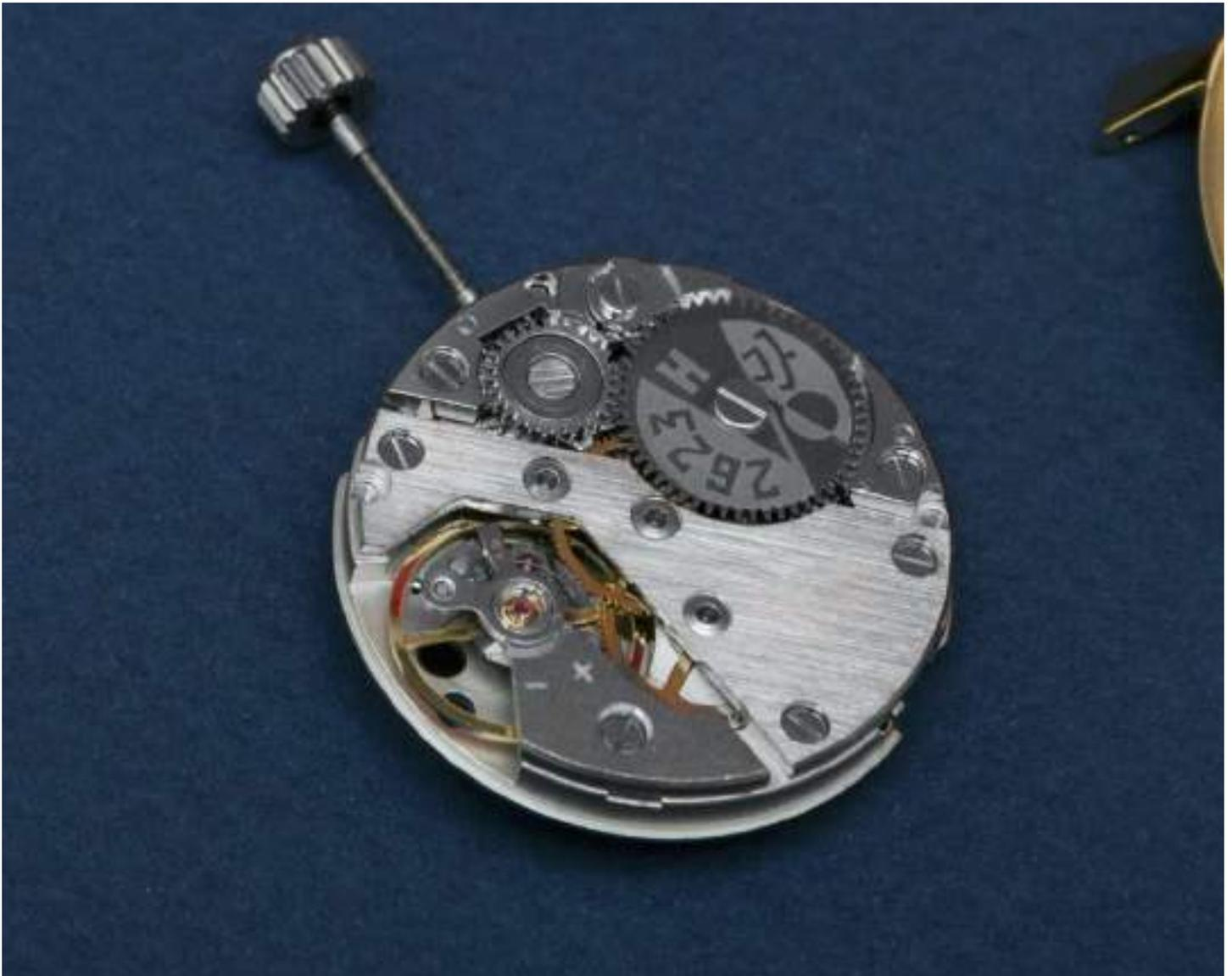
The Calibre 2623 is extremely close to what was found in the original 1970 watch. This hand-wound movement, with 24-hour display, is by no means a high-end, Haute Horlogerie piece. It was created to be robust, functional, easy to service and durable. This calibre runs at a slow frequency of 2.5Hz and boasts a 42-hour power reserve. It adjusted in 4 positions and should run at  $\pm 10$  seconds/day.
